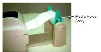
When the media roll has the inner core diameter of 76.2 mm (3"), use the 3"-Diameter Media Shaft included in the optional External Media Roll Hanger.
